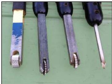
Detailing Tools: Knurling, texturing, spiraling and Pyramid.
